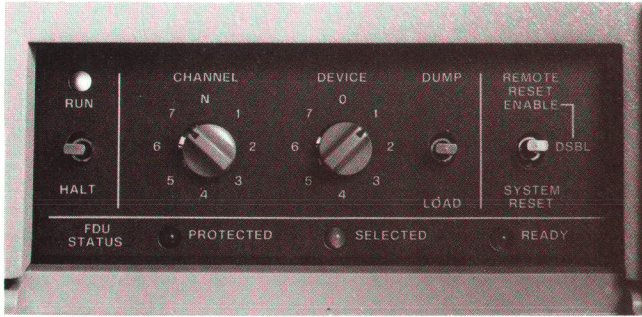
Fig. 3. HP 300 control panel is used when starting the system.
